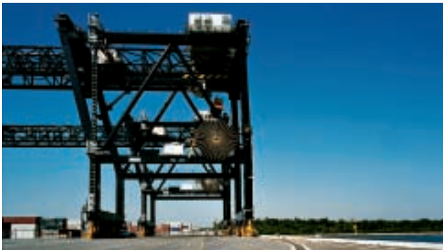
Pull & Store reels at work at Everglades terminal, USA
