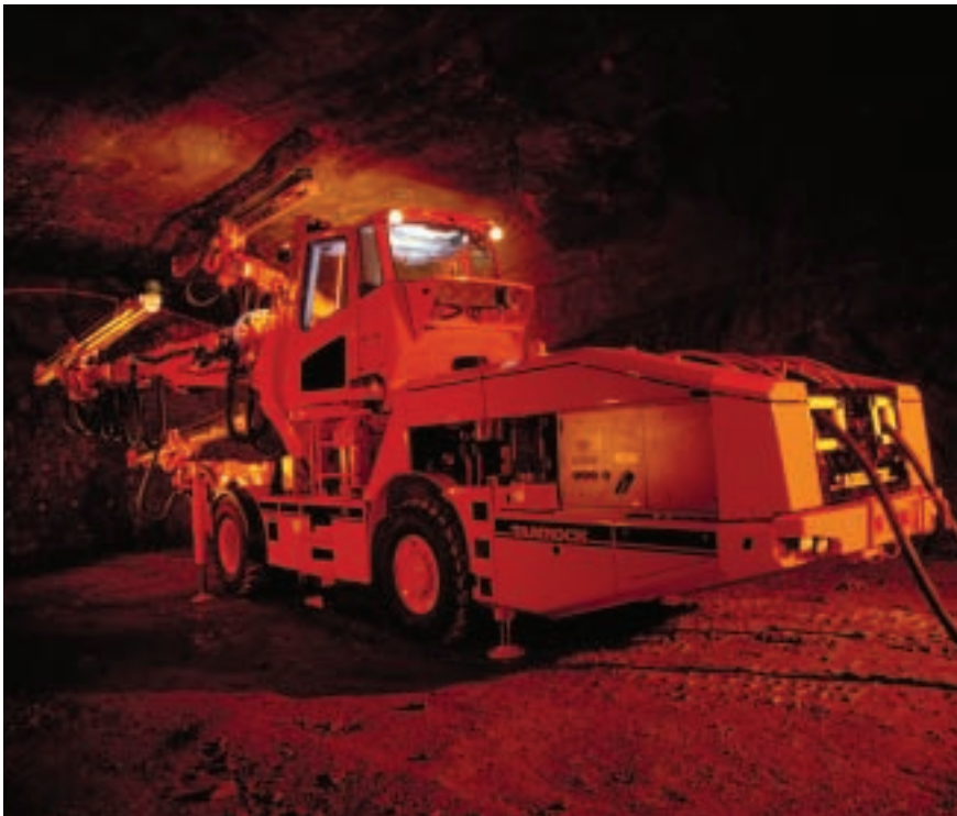
A Tamrock drill rig equipped with Cavotec Specimas cable and hose reels.
