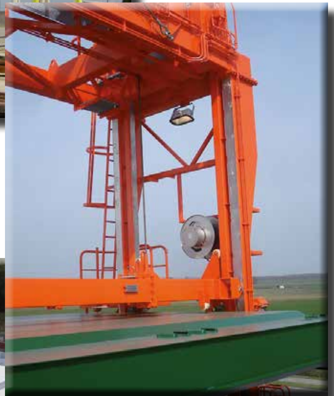
AV50 cable reel (stainless steel), feeding a portal crane on a freight ship
